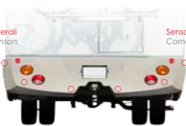
Sei sensori posteriori (due ai lati) Six rear sensors (two on the corners)
